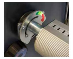
The front bottom axle (unwinding axle R1) and the rear axle (rewinding axle R2) are secured with a locking mechanism so that the axle remains securely in the holder.
