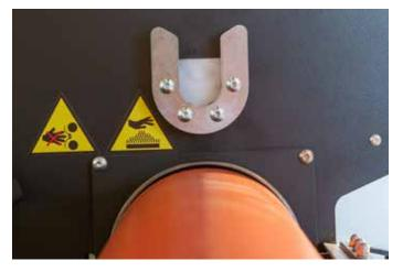
• The intake directly above the upper lamination roller can be used to place a roll of APP film directly onto the upper lamination roller.
