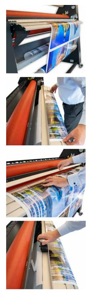
• You can load prints or laminated prints on a roll into the rear reel seat or move them sheet by sheet.
