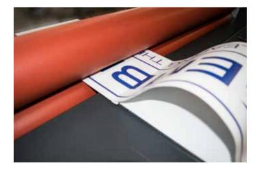
• Close the laminating rollers to secure the print and plate. The print should be longer than the plate.
