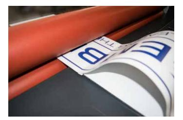
• Separate the first half of the backing paper from the self-adhesive print and start the lamination process.
