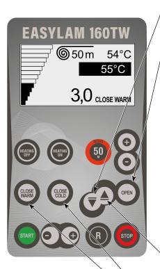
• Open the lamination rollers by pressing the key ▼ or "**OPEN**". (Fig. p. 5) and load the laminate as shown in the figure. Slide an empty roll core onto the rewind axle R3 (fig. p. 3 no. 6) so that the protective liner/cover paper can be wound up.
