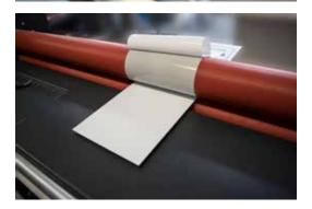
• Pull off 3 - 4 cm from the cover paper of the plate and fix the print on the plate by hand.
