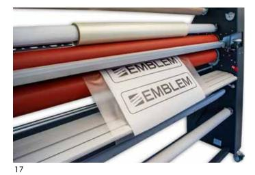
• Feed the weeded plot between the lamination rollers and apply the APP film by starting the lamination machine.
