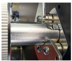
The drive pin is inserted into the guide of the axle.
