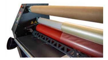
• Pull the APP film between the laminating rollers and apply the film with the laminator to weeded film plots.
